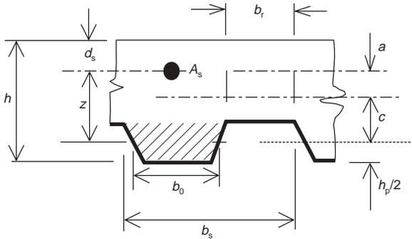
Fig. A.1. Model for stiffness of a composite slab in hogging bending
